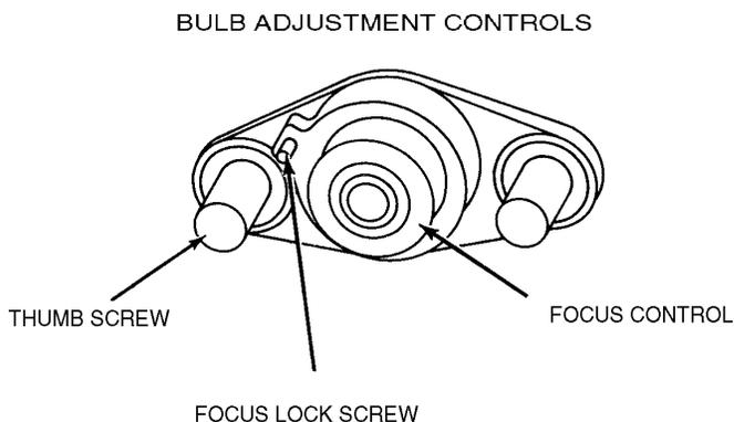
THE CENTER SECTION of the bulb positioning controls is a threaded member that focuses the bulb in relation to the reflector. Turning this adjustment moves the bulb in only one plane, into or away from the reflector. Turning this section clockwise moves the arc away from the reflector. The small knurled screw to the left of this section can be tightened to lock the focusing mechanism after the following procedures have been completed.
