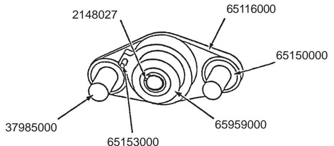
Fade Out & Heat Filter Assembly
