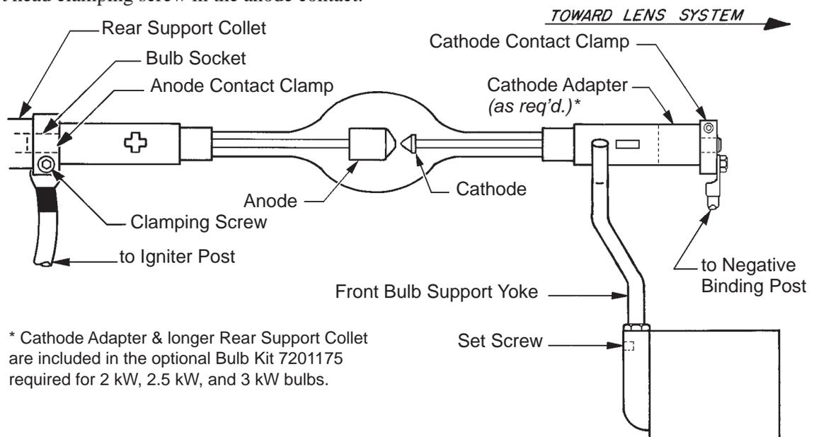
REST THE CATHODE END CAP in the “V” of the bulb yoke. Dress the bulb lead directly in front of the bulb support yoke to minimize the projected shadow, but do not allow it to touch grounded metal lamphouse components; the bulb yoke and the support casting are insulated from ground. Slide the cathode contact clamp over the cathode (-) pin and securely tighten the clamping screw.
