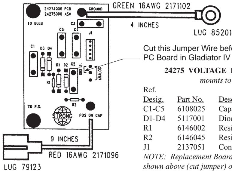
Cut this Jumper Wire before installing 24275
