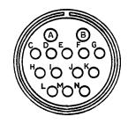
Modification for use with Spotlight or other non-console lamphouse: Remove the jumper from between Pin E & F; remove black lead from Pin C and relocate to Pin F. This will supply 110 V.AC to the main board for the **GO** light.
