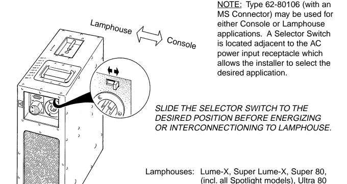
Male MS Connector optional on Motion Picture lamphouse cables
