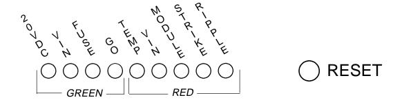
WHEN ALL FOUR of the green indicator lights are glowing, the power supply is operating trouble-free. One or more red lights, when glowing, indicates that a problem exists, and disables operation of the power supply. The red light(s) latches and remains glowing until the RESET button is depressed after the problem has been corrected.
