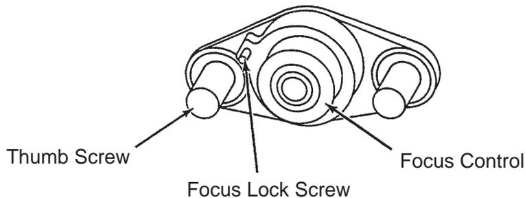
THE FOLLOWING METHOD is recommended to position the xenon bulb inside the reflector in order to project the best light to the stage.
