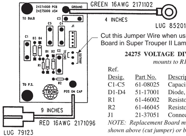
Cut this Jumper Wire when using 24275 PC Board in Super Trouper II Lamphouse
