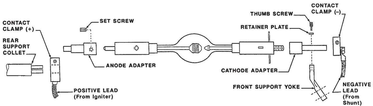
**NO ADAPTERS REQUIRED FOR 2000 WATT TYPE "HS" BULB**
