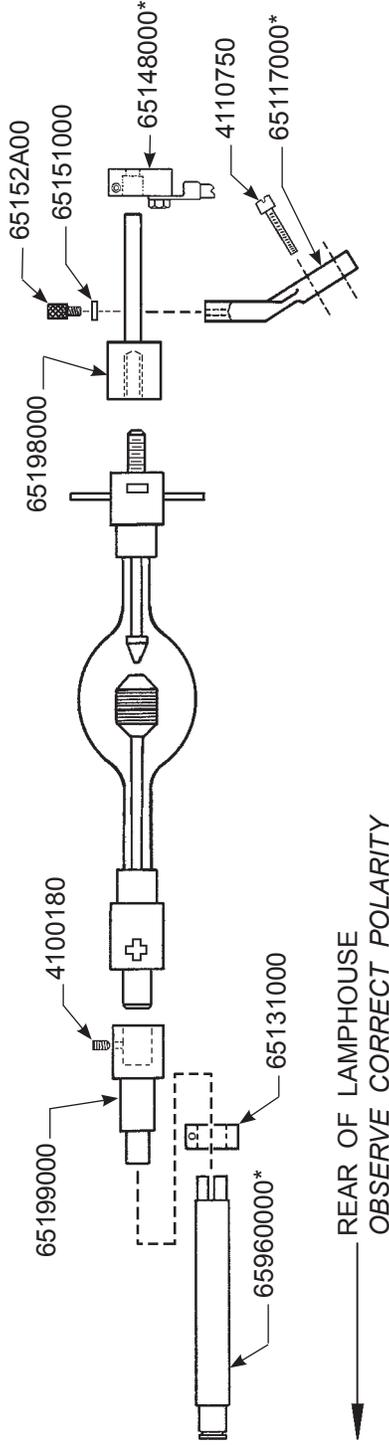
\* Replace Collet, Front Bulb Support, and Cathode Clamp before installing bulb.
